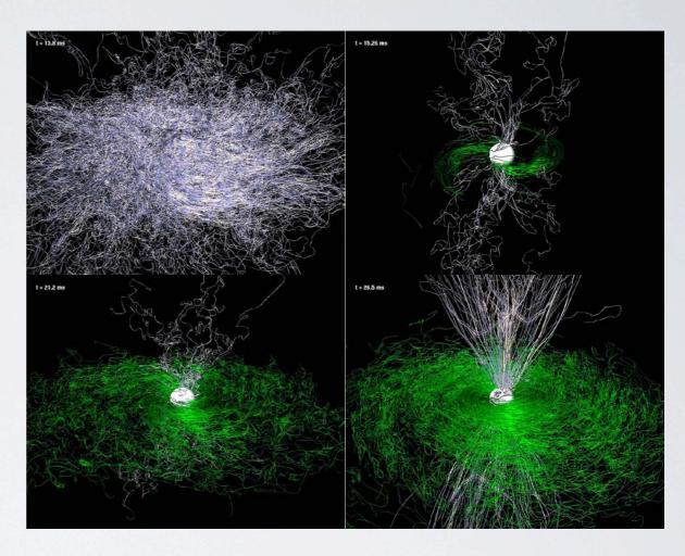
Some results of our simulations are presented in the figures, which show the magnetic-field lines (white lines in the equatorial plane and green lines outside the disc) at selected times.
