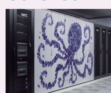
Type: Scalar **OS**: Linux # of nodes: 319 Peak performance: 1.463 Pflops Interconnect: InfiniBand EDR
