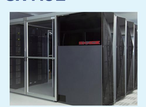
**Type:** Vector OS: Super UX # of nodes: 1536 # of cores: 6144 Peak performance: 423 TFlops
