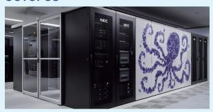
OCTOPUS means Osaka university Cybermedia cenTer Over-Petascale Universal Supercomputer. OCTOPUS is a cluster system supposed to start its operation in December 2017. This system is composed of different types of 4 clusters, General purpose CPU nodes, Xeon Phi nodes, GPU nodes and Large-scale shared-memory nodes, total 319 nodes. These nodes and large-scale storage "EXAScaler" (Lustre 3.1 PB) are interconnected on InfiniBand EDR (100 Gbps) and form a cluster.
