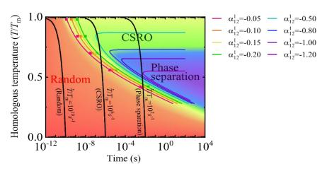
TTC diagram for the quinary model HEA. Dots indicate data directly obtained by kMC and the colored lines are the fitting results of the data. Larger CSRO parameters ( $\alpha_{12}^1$ ) values imply phase separation. The solid black lines show temperature changes at constant quenching rates.
