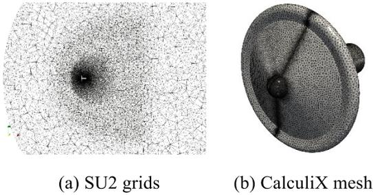
Fig. 2: Grids for fluid and structural analysis
