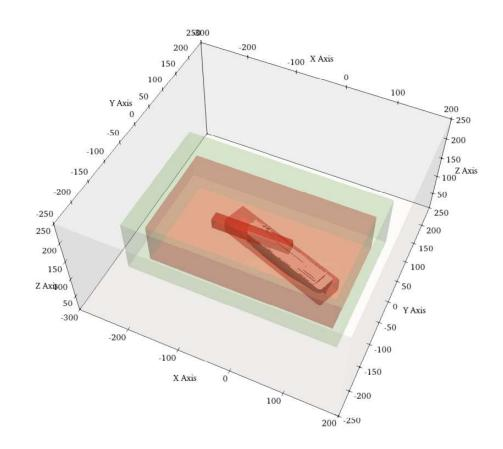
Fig. 2 Mesh refinement domain used for the case
